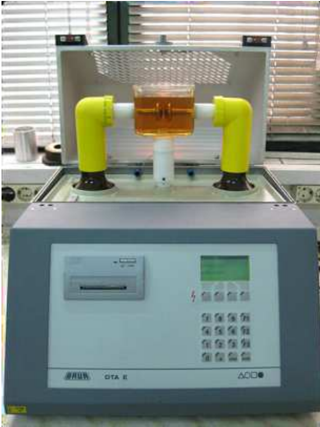
Fig. 1: Device for the measurement of dielectric strength
