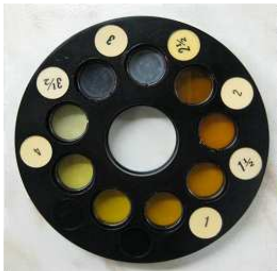
Fig. 4: Typical glass colored disc
