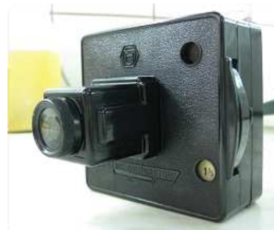
Fig. 3: Chromometer Hellige Comparator
