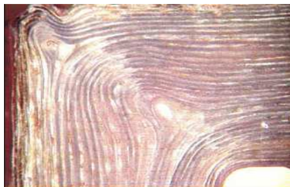
Fig. 2: Imperfections of winding insulation at the edges (after [10])
