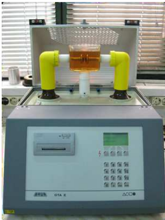
Fig. 1: The test cell for breakdown voltage measurements
