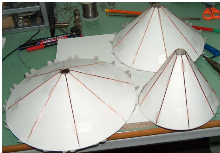
Fig. 14: Constructed frustum cones for \alpha = 60^\circ, 90^\circ, 120^\circ
