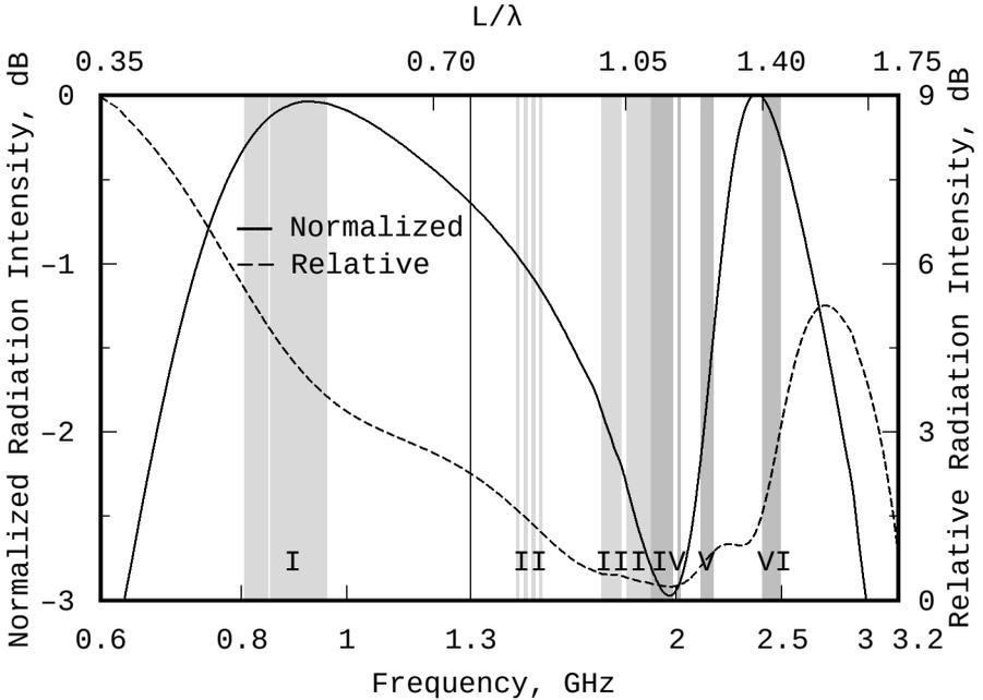
Fig.4: Predicted radiation intensity on horizontal plane.
