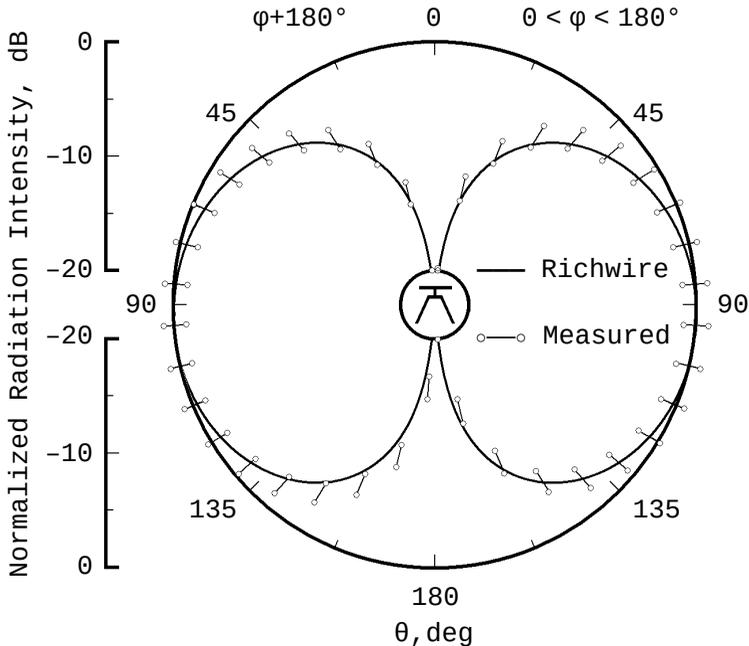
Fig.6: Measurement error bounds on a vertical plane
