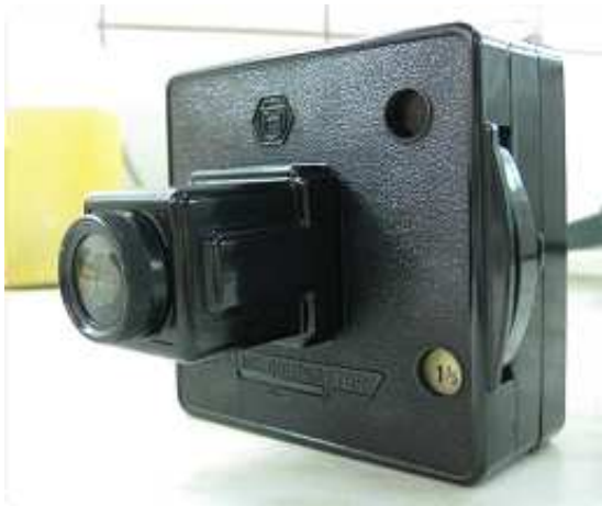
Fig. 3: Chromometer Hellige Comparator
