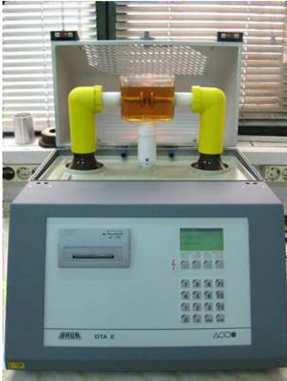
Fig. 1: The test cell for breakdown voltage measurements
