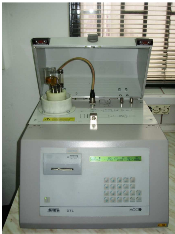
Fig.2: Device for measurement of \tan\delta and resistivity
