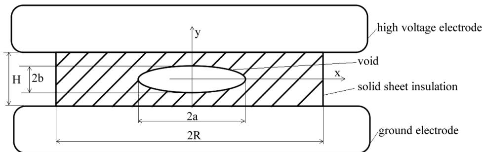
Fig. 2: Cross section of insulation with a void
