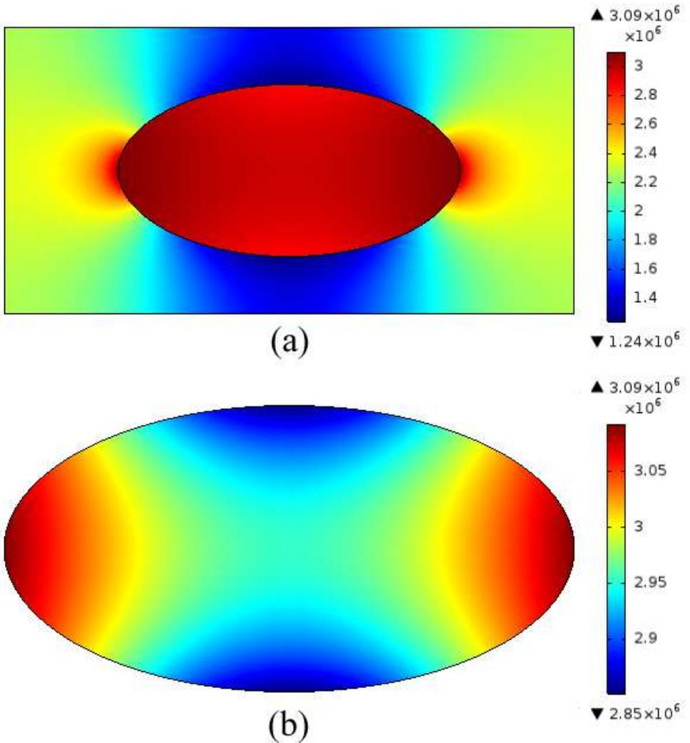
Fig. 3: Electric Field Distribution under IV in AC Case
