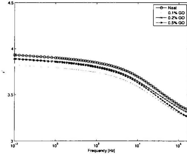
Fig. 9 Dielectric constant epoxy nanocomposite with GO at 20<sup>o</sup> C
