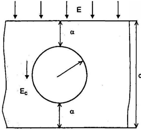
Fig. 11 Enclosed cavity in a solid dielectric
